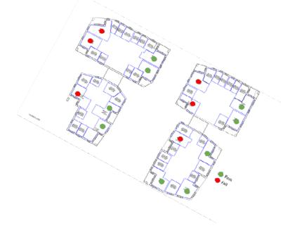
Fig 7 - Showing location of sunlight BRE pass/fails at second floor level
